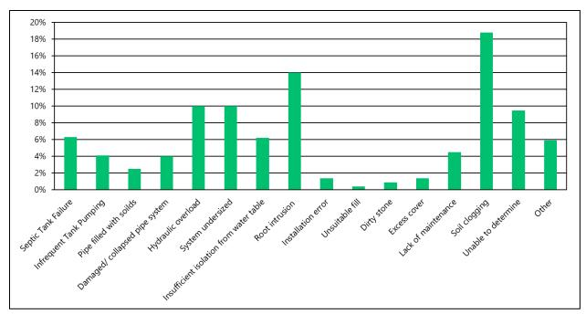
**Figure 116.** Probable cause(s) of failure of failed systems 2013 - 2015 SOURCE: Michigan Statewide Failed Sewage System Evaluation Summary Reports from 2013 - 2015, MDEQ.
