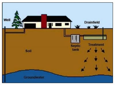
*Figure 112. Typical septic system SOURCE: MSU, Institute for Water Research, 2007.*
