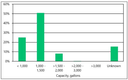
Figure 113. Septic tank capacity of failed systems 2013 - 2015
